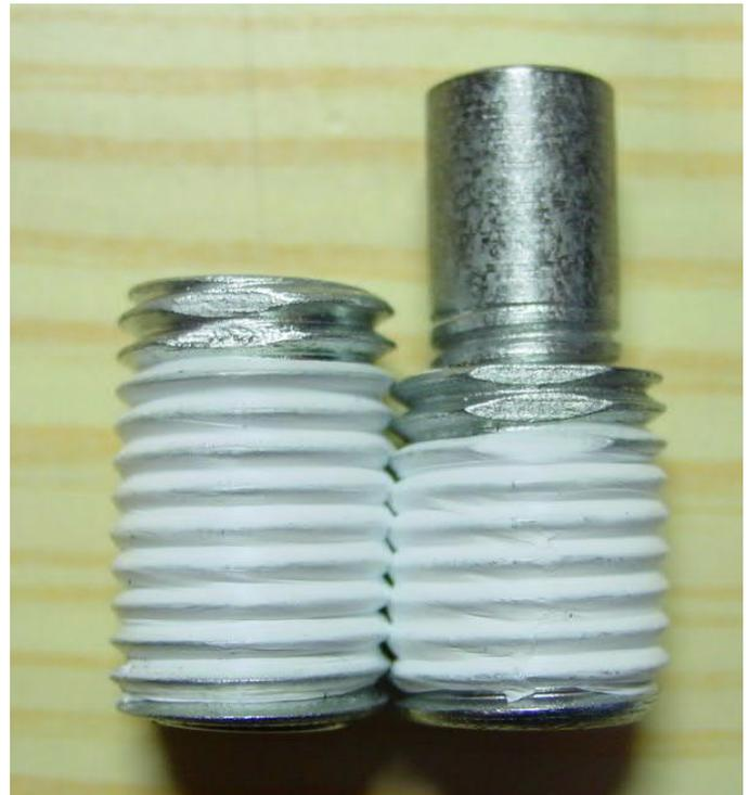
You have to wrap only 3-4 times if both connector parts were tight during the first adjustment.
